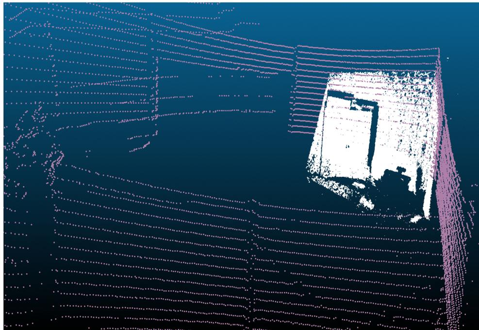
**Figure 6.** Alignment of cloud points LiDAR of RealSense L515 camera (white) to the cloud point of the Vehicle LiDAR (purple).
