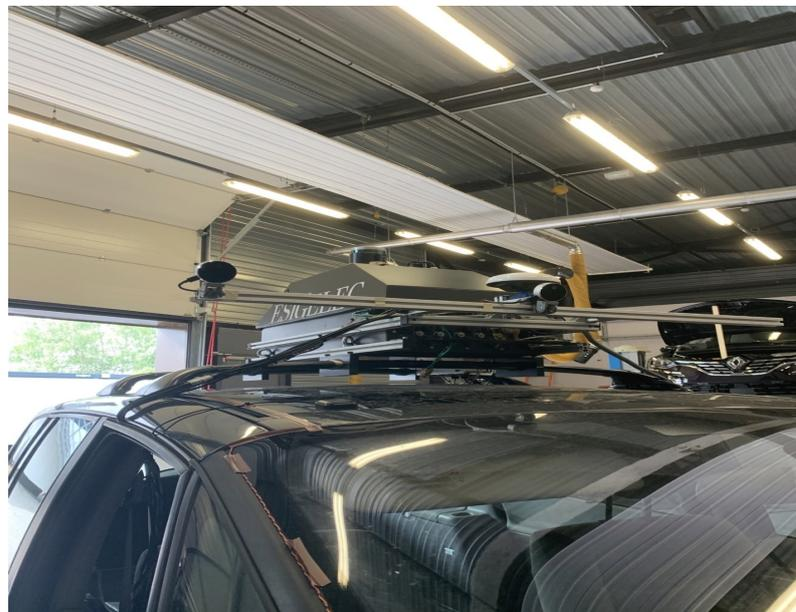
**Figure 5.** The instrumentation of the camera on the roof of the vehicle. The camera is fixed on a rail just in front of the LiDAR.
