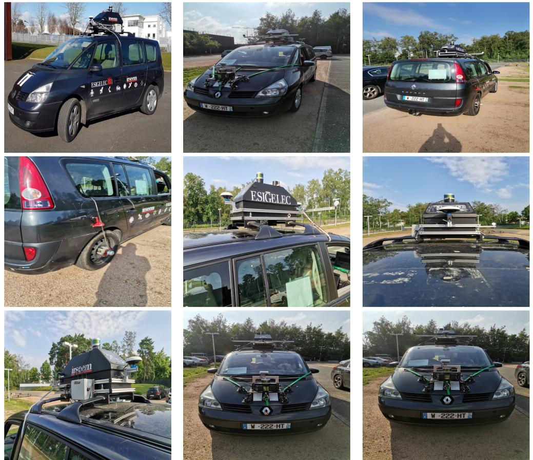
**Figure 3.** Instrumented IRSEEM Vehicle for data collection in smart mobility. The car trunk on the roof of the vehicle includes the whole sensors (Cameras, GPS/IMU, LiDAR, RADAR, Odometer). The odometer sensor is instrumented on the right rear wheel.
