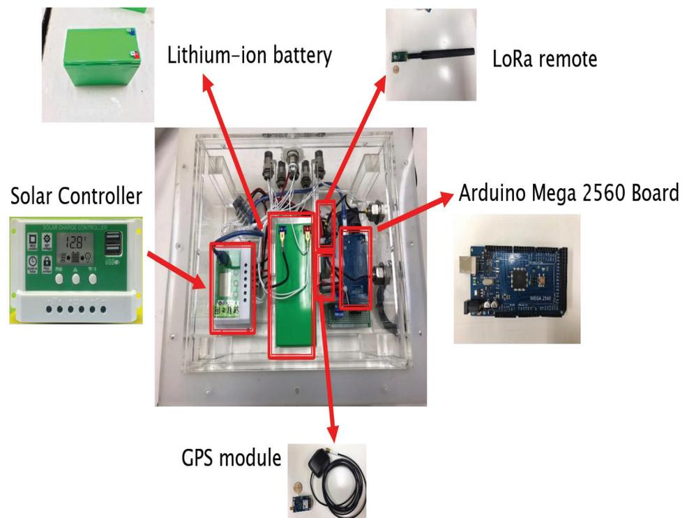
**Figure 4.** Control box of the proposed AI buoy.
