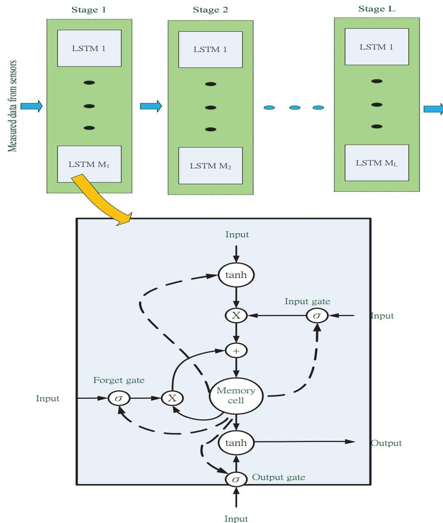
**Figure 5.** The multilayer architecture and cell structure of long short-term memory (LSTM).
