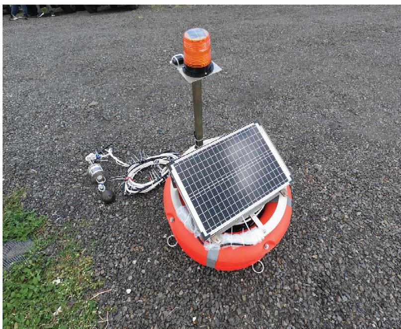
**Figure 2.** Proposed offshore buoy: main body and flow sensor tube.
