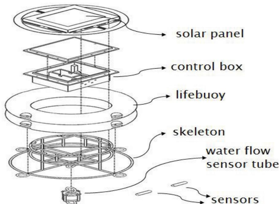
**Figure 1.** Architecture of the proposed offshore buoy.
