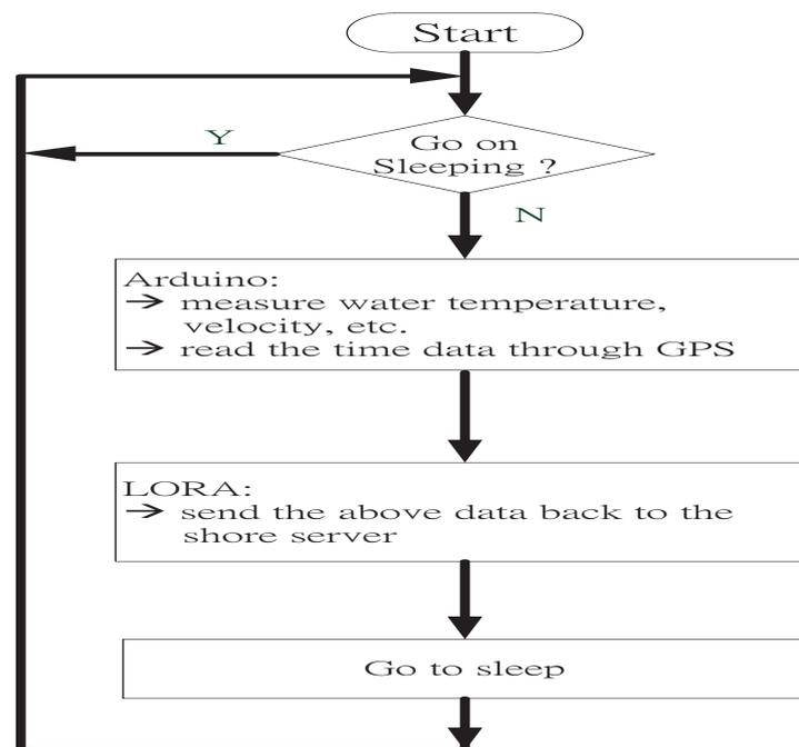
Figure 3. Operation flow of the proposed buoy.
