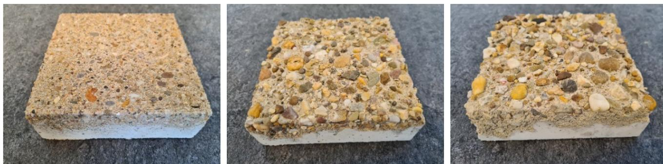
**Figure 5.** Overview of the three concrete specimens used as investigation objects for accuracy evaluation—to the left specimen 1 with 1.5 mm washout depth, in the center specimen 2 with 3.0 mm washout depth and to the right specimen 3 with 6.0 mm washout depth.
