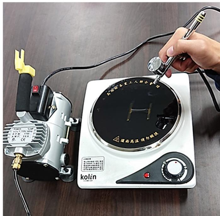
Figure 1. Experimental setup of gun spray deposition.
