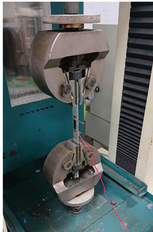
**Figure 12.** Al specimen subjected to tensile loading.
