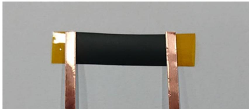
Figure 3. Strain sensitivity test specimen.
