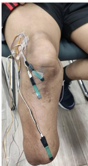
**Figure 3.** An example of force sensing resistor sensor placement on a residual limb.
