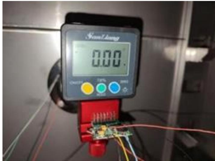
**Figure 12.** Accelerometer zero random drift test process.
