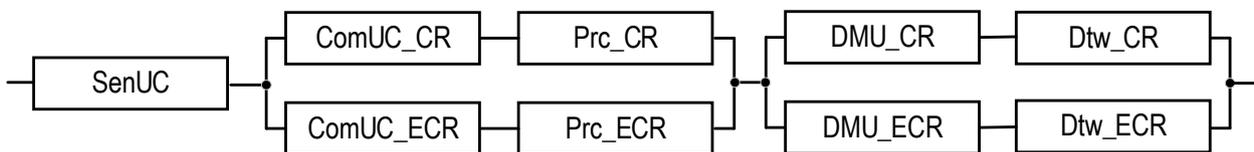
**Figure 5.** RBD that is utilized to calculate the reliability functions of systems  $S_{2,2}^{UC-N}$  and  $S_{2,2}^{UC-E}$  using Equations (5) and (6), respectively.
