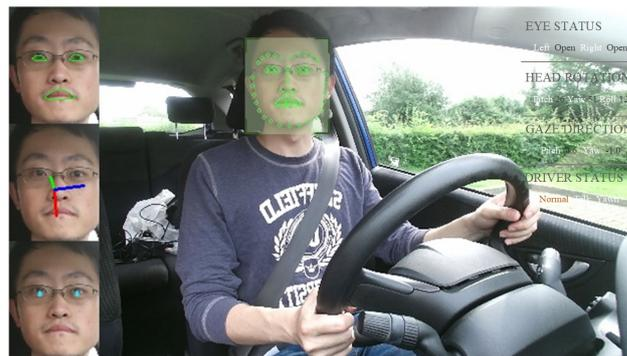
**Figure 1.** Example of our multi-state driver monitoring system.
