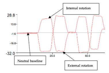
**Figure 2.** Estimating hip range using the smartphone (**left**) and the 3D motion capture (**right**). To calculate the maximum hip range the neutral baseline angle was subtracted from the maximum internal or external rotation values.
