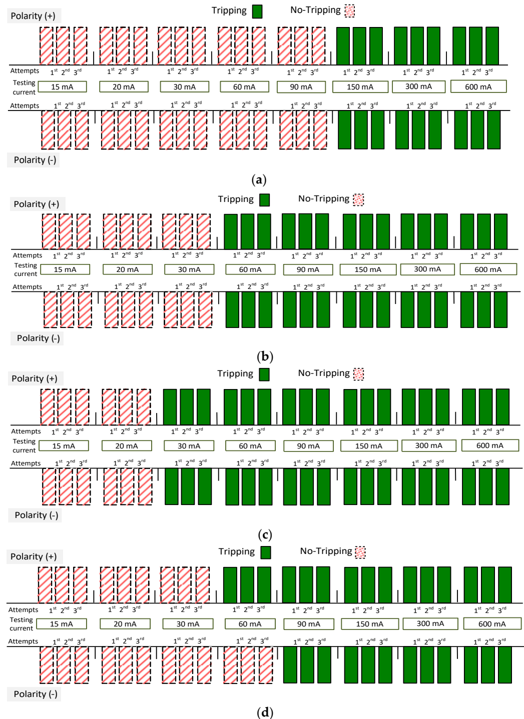
Figure 21. Tripping of the 30 mA A-type RCDs for a pure direct current (suddenly applied) of values 15, 20, 30, 60, 90, 150, 300 and 600 mA. Tested RCDs: (a) (RCD30_6); (b) (RCD30_7); (c) (RCD30_1); (d) (RCD30_8).
