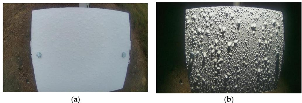
**Figure 5.** Example images of the reference surface: (a) color image acquired during normal daylight conditions and (b) color image acquired during the nighttime with the help of artificial illumination.
