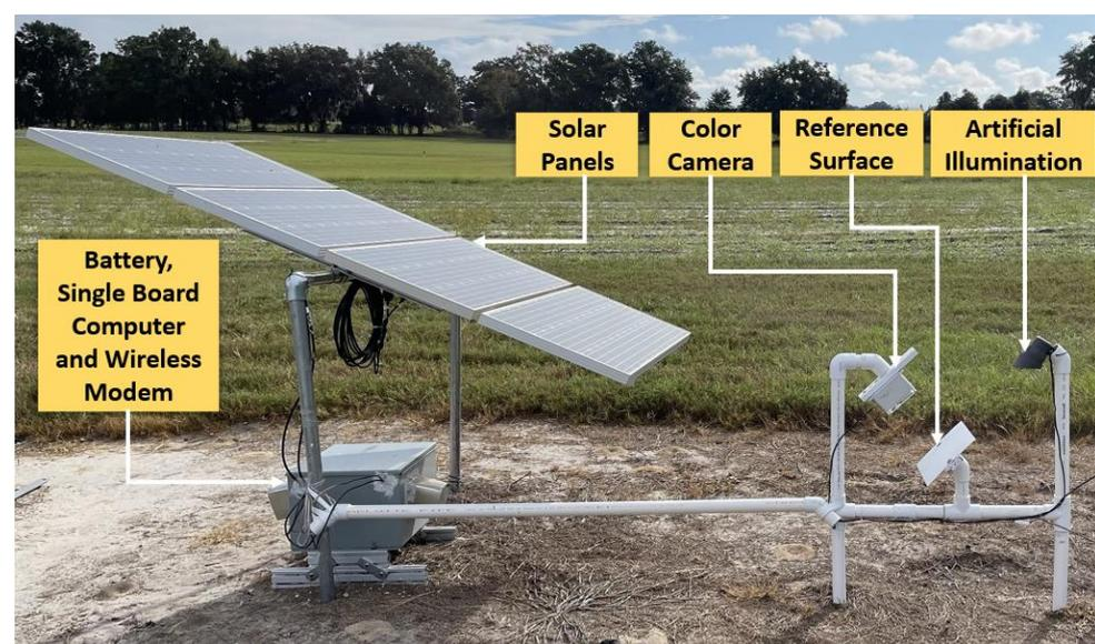
Figure 1. System to monitor a reference surface using an RGB camera at UF PSREU, Citra.
