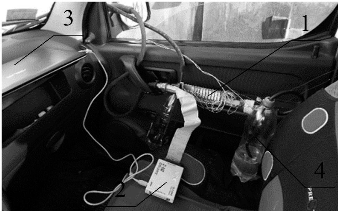
**Figure 4.** Carrying out experimental studies on the vehicle: 1, flowmeter; 2, analog–digital converter; 3, computer; 4, vessel with fuel.
