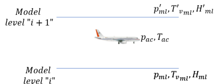
Figure 7. Computation of reference surface values and temperature lapse rate for estimating the barometric altitude from a pressure and temperature measurement at aircraft.
