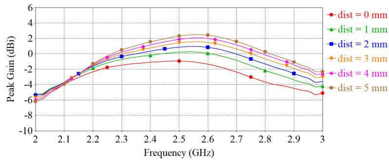
Figure 15. Peak gain vs. frequency when varying the separation between the antenna and phantom.
