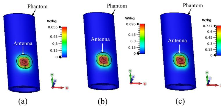
Figure 18. SAR distributions in the forearm phantom at: (a) 2.4 GHz, (b) 2.45 GHz and (c) 2.6 GHz.
