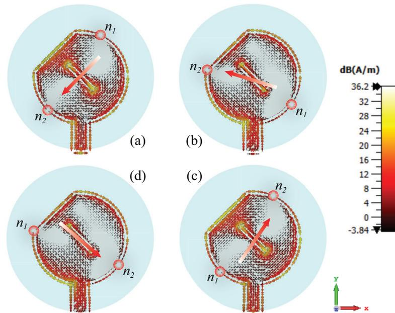
**Figure 2.** Surface current distribution of the antenna at 2.4 GHz at the time phases (a)  $0^\circ$ , (b)  $90^\circ$ , (c)  $180^\circ$  and (d)  $270^\circ$ .
