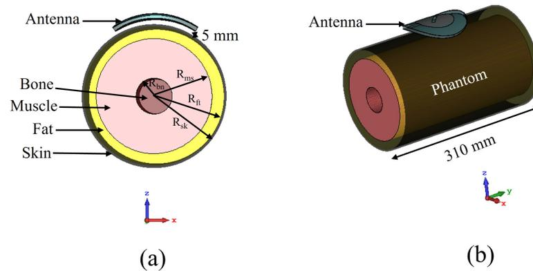
**Figure 19.** Antenna on top of the multilayer phantom: (a) cross-sectional view, (b) perspective view. ( $R_{bn} = 12.5$  mm,  $R_{ms} = 40$  mm,  $R_{ft} = 48.5$  mm,  $R_{sk} = 50$  mm).
