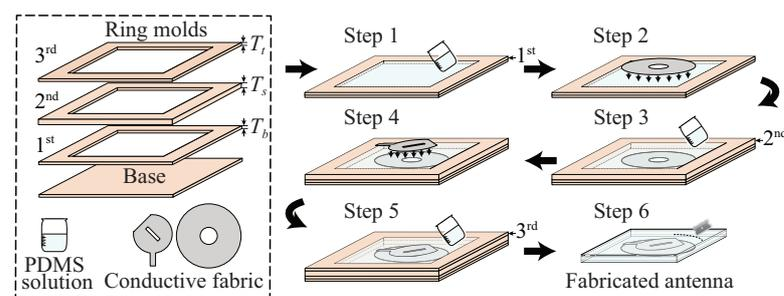
**Figure 12.** Schematic representation of the antenna fabrication process.
