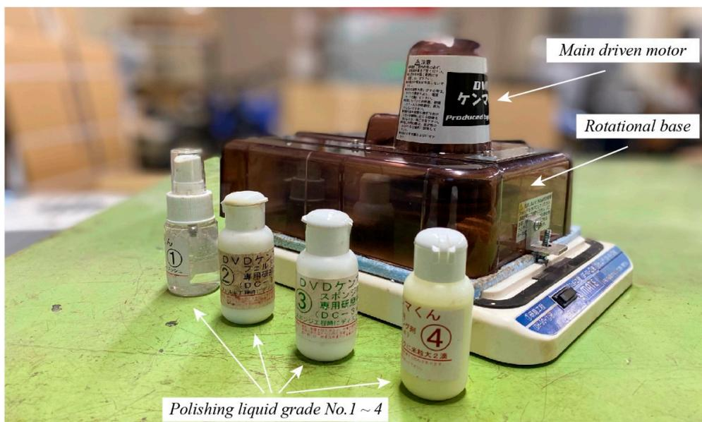
Figure 5. A self-configured plastic gear polisher. Originally, this is a DVD polisher by Kenmac.
