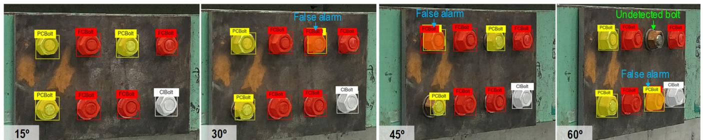
**Figure 13.** Visualization of corroded bolt detection results at different capturing angles.
