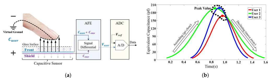
**Figure 2.** Using the capacitive sensors in a touchscreen, BioTouch continuously authenticates users according to their bio-capacitance during finger touching. (a) The collection of equivalent capacitance ( $C_{user}$ ). (b) The change of equivalent capacitance ( $C_{user}$ ) during touching.
