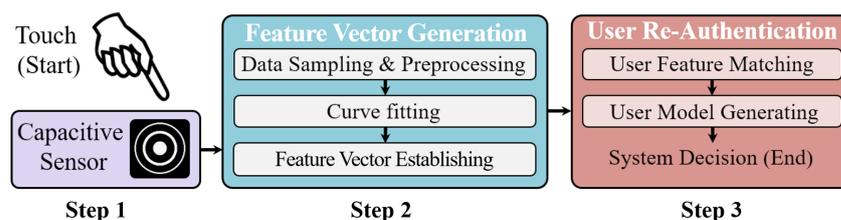
**Figure 1.** During touching operation, BioTouch transparently verifies the current user's legitimacy through the following three steps: Combined user feature collection (Step 1, Section 4), user feature vector generation (Step 2, Section 5) and user re-authentication (Step 3, Section 6).
