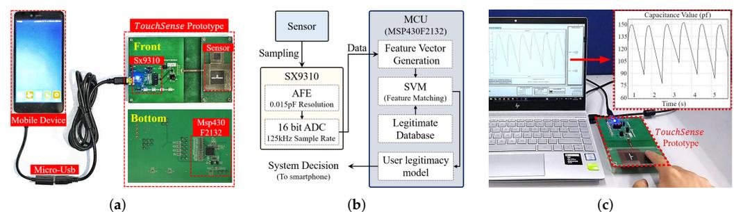
**Figure 7.** BioTouch contains a novel designed PCB to control the device. We can also use a laptop to monitor the working states of the prototype, where the sensed capacitance value is shown in the window in real time. (a) BioTouch prototype. (b) Prototype block diagram. (c) Working status monitoring of BioTouch.
