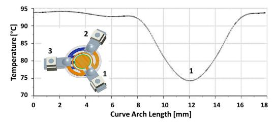
Figure 5. Temperature profile on the electrode edge.
