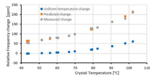
**Figure 12.** Comparison between the relative frequency changes predicted by the model and the measured ones.
