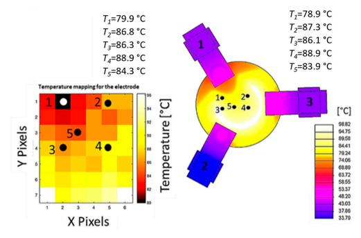
**Figure 8.** Temperature map on the electrode: comparison between the measured thermal image (**left**) and the model predictions (**right**).
