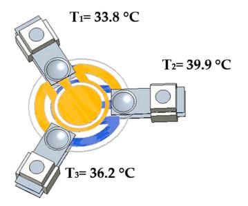
Figure 3. Temperatures of the supports' spacers.
