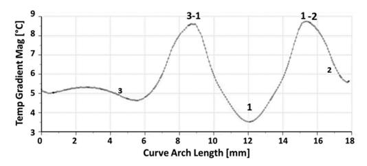
Figure 6. Temperature gradient magnitude on the electrode edge.
