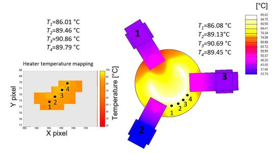
**Figure 9.** Temperature map on the heater: comparison between the measured thermal image (**left**) and the model predictions (**right**).
