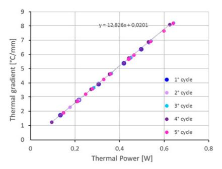
Figure 13. Temperature gradient vs. power dissipation.
