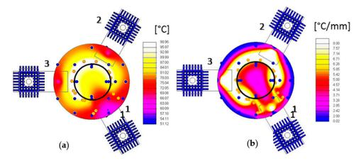
Figure 4. (a) Electrode temperature mapping; (b) Temperature gradient.
