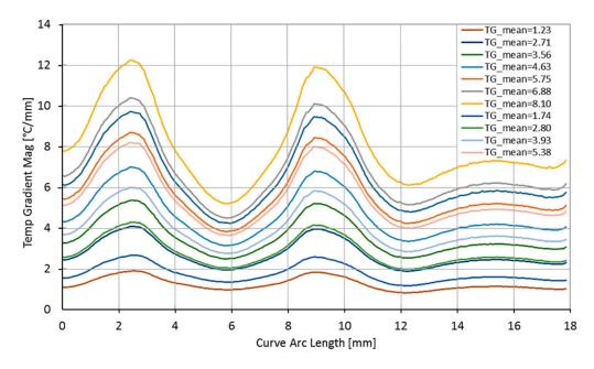
The thermal gradients were evaluated for different power dissipations of the heaters and used to assess the effects on the crystal frequency are shown in Figure 10.
