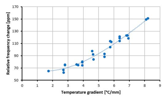
Figure 11. Frequency variation vs. thermal gradient.
