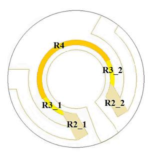
Figure 2. Different heater areas for power distribution.
