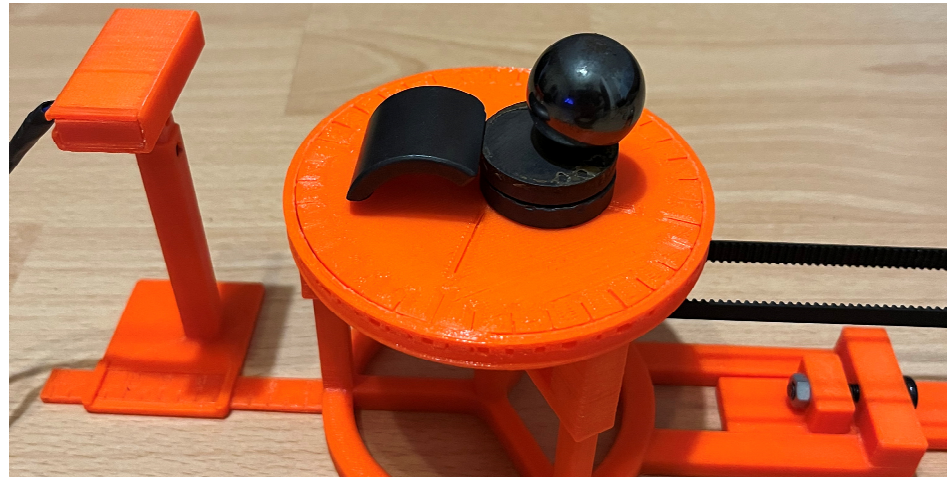
Figure 21. A system of several permanent magnets used during measurements of an irregular magnetic field.
