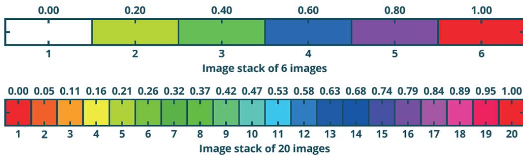
**Figure 2.** Correlation between hue and number of images in the stack—based on [8].
