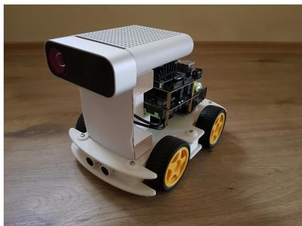
**Figure 3.** Ground robot used to record the real-world dataset. An OpenBot equipped with an Azure Kinect RGBD camera.
