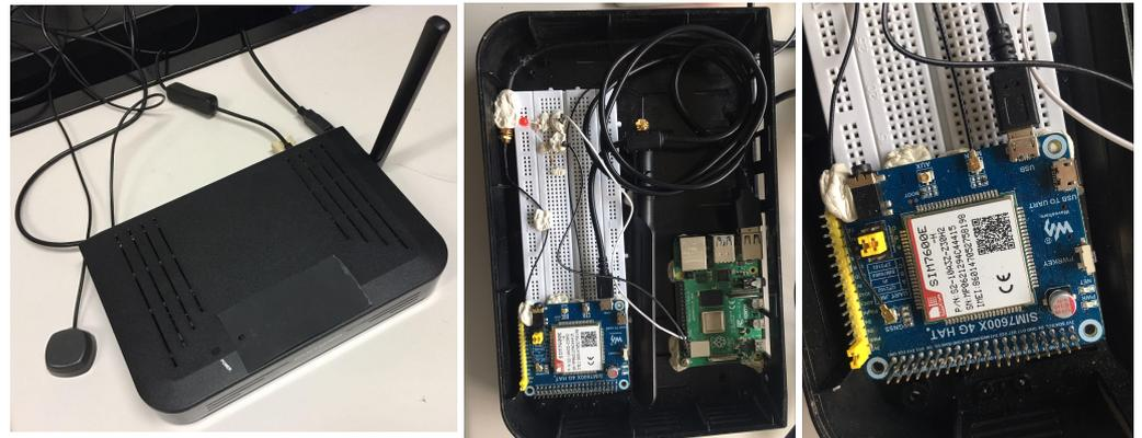
**Figure 4.** Prototype of the WiFi scanner with external BrosTrend AC650 WiFi antenna (left); the Raspberry Pi4 with LTE antenna and 4G hat (center); the SIM7600X 4G hat (right).
