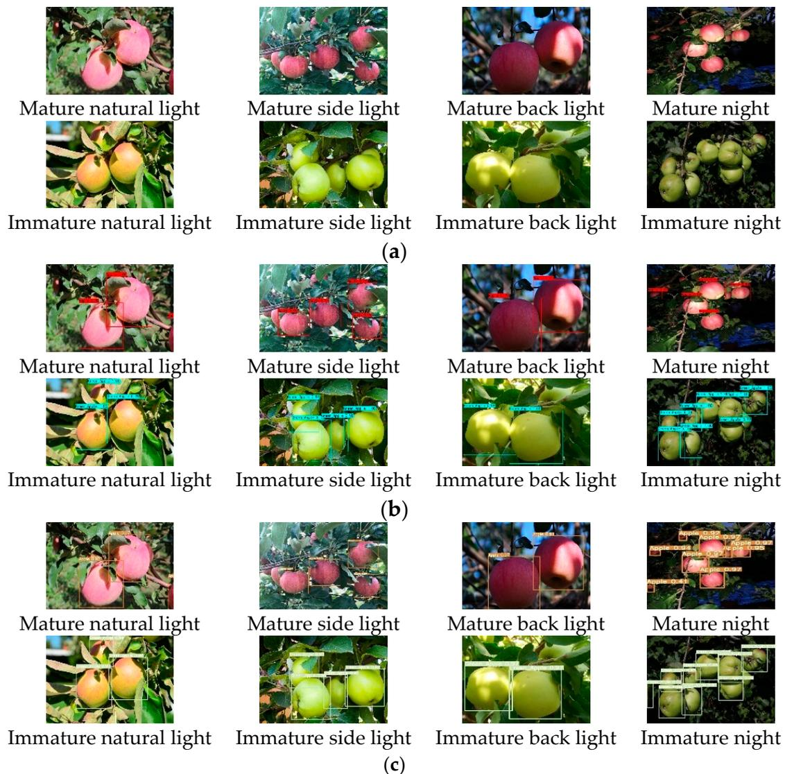
**Figure 10.** Detection effect of apples under different illumination before and after YOLOv5 improvement. (a). Original picture; (b). YOLOv5; (c). Improved YOLOv5.
