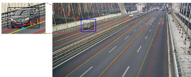
Figure 8. Mismatch between the bounding box and lane.
