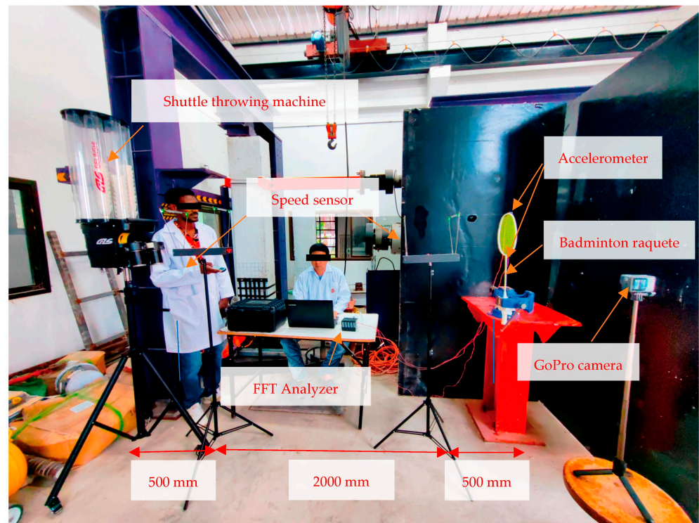
Figure 3. Experimental setup and shuttlecock shooting arrangement.
