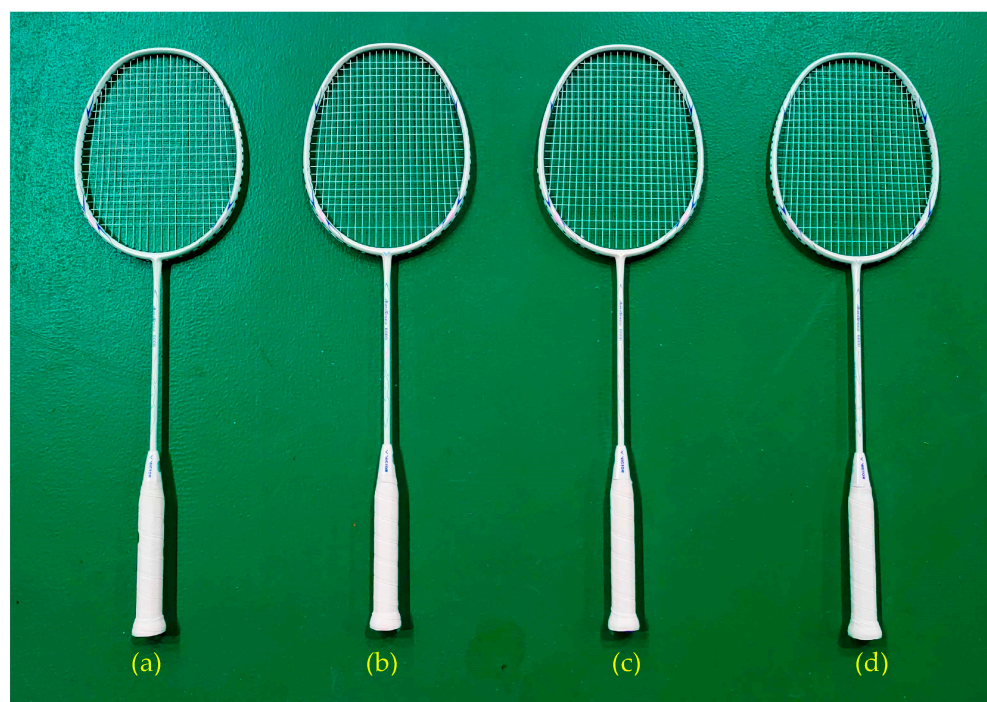
Figure 1. Carbon graphite mixed epoxy resin badminton frame (Victor model ARS-6000A) with different string patterns: (a) type A; (b) type B; (c) type C; (d) type D.
