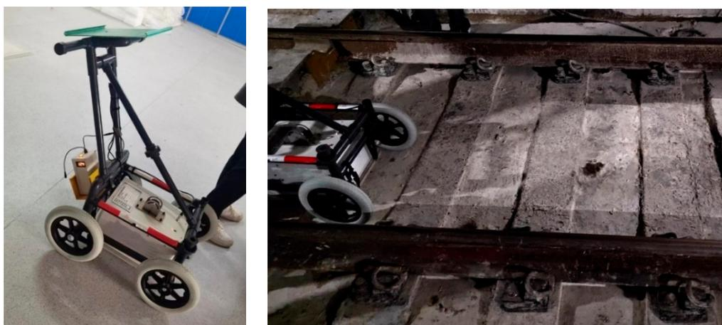
**Figure 1.** Ground-Penetrating Radar Vehicle TGRI-GPR.
