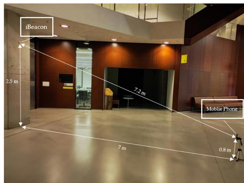
**Figure 15.** Testbed for iBeacon Localization Field Experiment in the Large Area.
