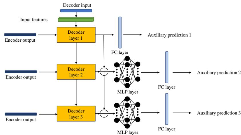
**Figure 4.** Demonstration example of the three-layer feature fusion decoder of TCF-Trans.  $\oplus$  donates feature fusion operations.
