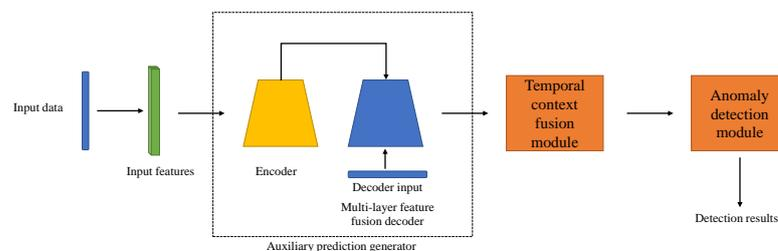
**Figure 3.** Block diagram of overall structure of TCF-Trans.
