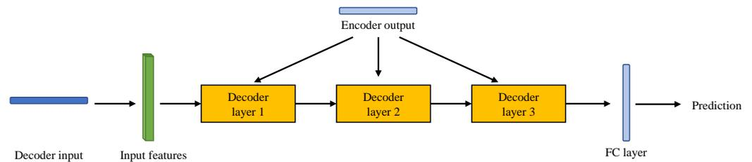
**Figure 1.** Demonstration example of the 3-layer decoder block diagram for the original Informer network.
