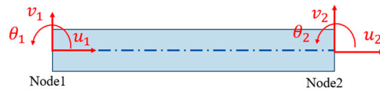
Figure 7. Plane beam element.
