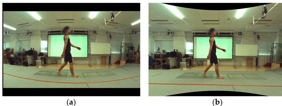
**Figure 3.** Lens distortion correction by Vicon Nexus version of 2.10. using calibration information from the Vicon system. (a) Pre-correction; (b) post-correction.
