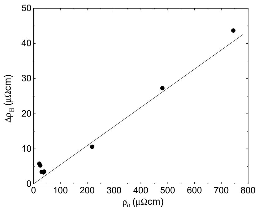
**Figure 5.** The hydride scattering resistivity term  $\Delta\rho_H$  as a function of resistivity for films of different thicknesses. A solid line is a guide to the eye.
