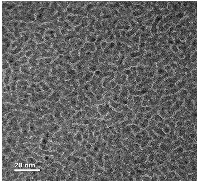
**Figure 2.** TEM micrograph of the 5 nm thick Pd film. Pd is dark.
