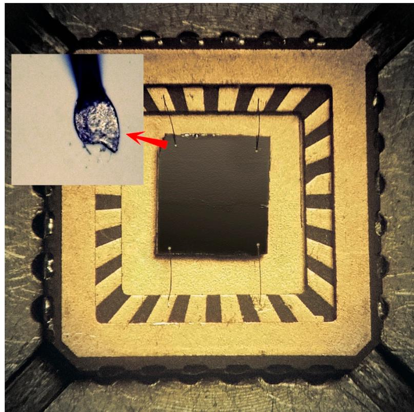
**Figure 1.** Image of  $5 \times 5$  mm sample mounted in the sample holder. Al/Si wires are attached by bonding.
