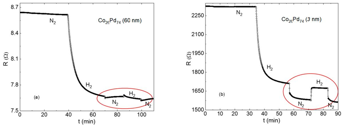
**Figure 6.** Resistance response of 60 nm (a) and 3 nm (b) thick  $\text{Co}_{26}\text{Pd}_{74}$  films to the sequences of hydrogenation and dehydrogenation cycles. The H scattering terms are marked by ellipses. The background resistance decrease is due to a gradual thickness expansion in the hydrogen atmosphere.
