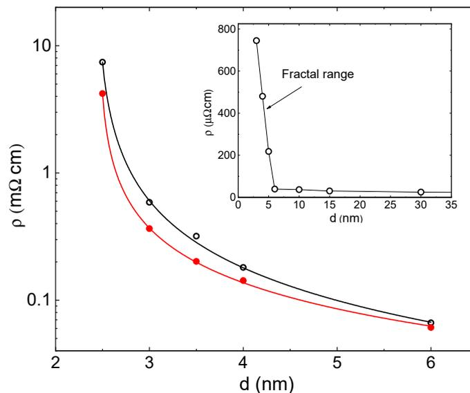
**Figure 3.** Resistivity of Pd films as a function of thickness prior (open circles) and after (solid circles) hydrogen loading. Solid lines in the main frame fit to Equation (2):  $\rho(d) = \alpha\rho_0(d - d_c)^{-m}$ .  $d_c = 2.4 \pm 0.05$  nm and  $m = 1.1 \pm 0.1$  in both states. Inset: resistivity as a function of thickness prior to hydrogen loading in a linear scale.
