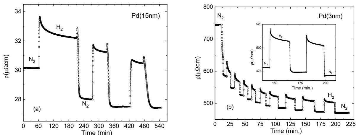
**Figure 4.** Resistivity response of 15 nm (a) and 3 nm (b) thick Pd samples to the sequences of hydrogenation and dehydrogenation cycles (sequential exposure to 1 atm 4% H<sub>2</sub>/N<sub>2</sub> gaseous mixture followed by N<sub>2</sub>). The sharp increase in resistance on hydrogen loading and the respective drop on hydrogen removal are due to the hydrogen scattering.
