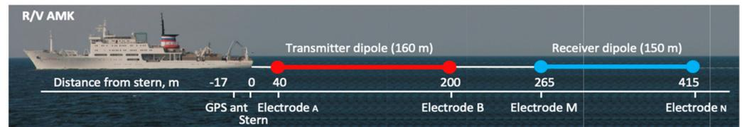
**Figure 6.** Typical configuration of the towed electrical array used in marine surveys for TDEM acquisition.
