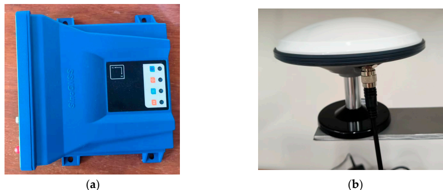
Figure 1. Main equipment of data collection: (a) M900SE receiver; (b) AT60 antenna.
