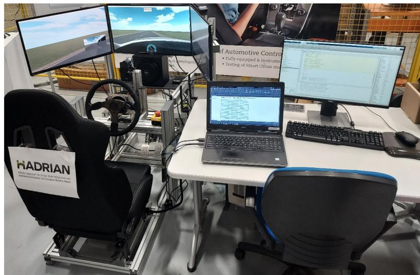
**Figure 3.** Driving simulator setup for the user tests.
