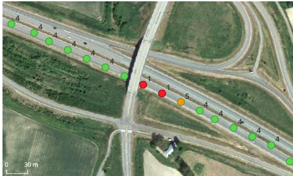
**Figure 2.** Example of the effect of bridges over the road. The car trajectory is marked with colored and labeled dots indicating the solution type in each epoch, as follows: SPP (red, 1), RTK-float (orange, 5) and RTK-fix (green, 4).
