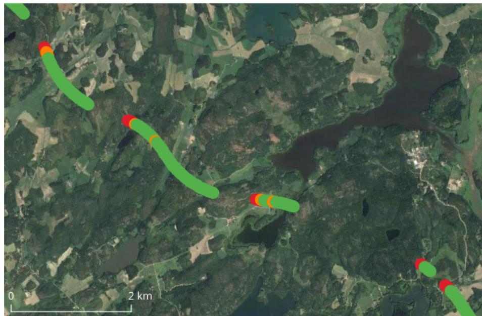
**Figure 3.** Example of tunnel types encountered in the highway. The figure shows five in a row (discontinuities of the dots). The red dots (SPP solutions) mark the exit of the tunnels.
