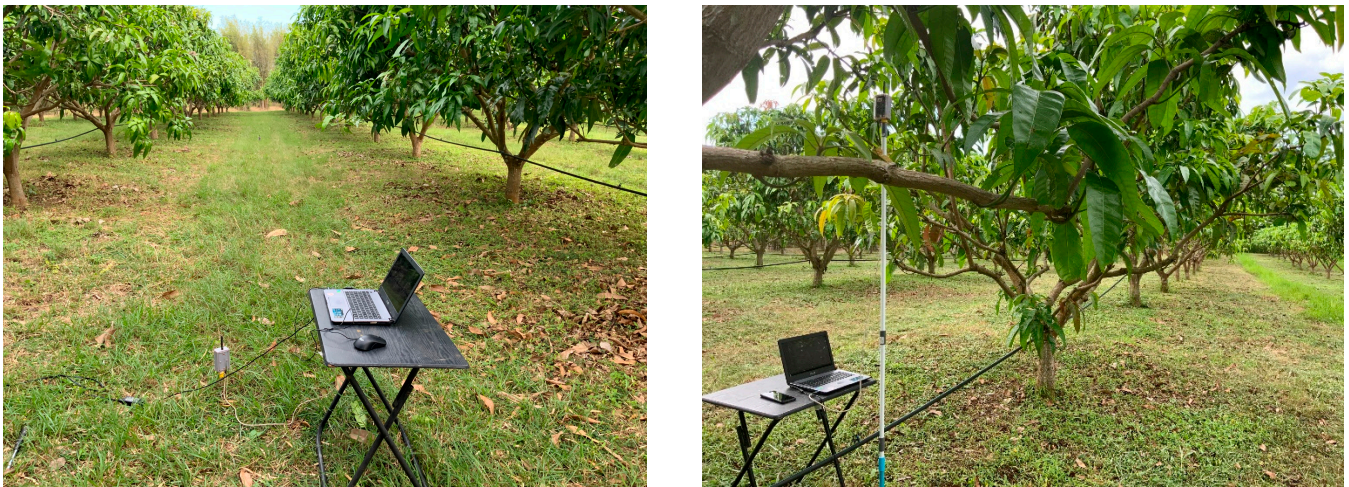
Figure 2. RSSI measurement for LOS (left) and NLOS (right).
