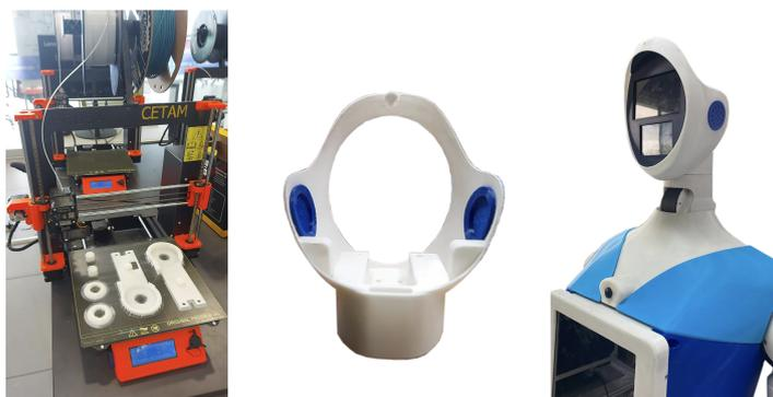
**Figure 4.** The manufacturing process of the Qhali robot.
