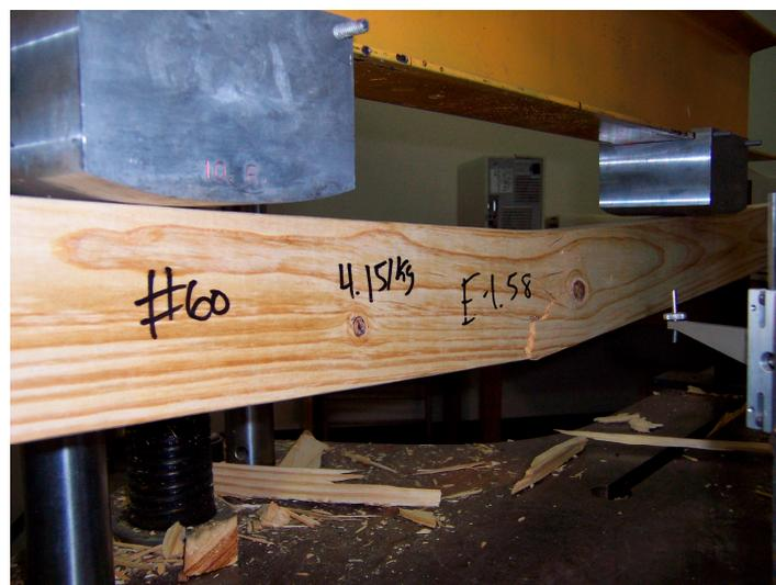
Figure 1. Destructive testing of a  $2 \times 4$  lumber in edgewise bending as per ASTM standards.
