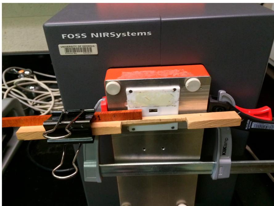
**Figure 2.** Acquisition of diffuse reflectance near-infrared spectral data from a wood sample on a FOSS NIRSystems Model 5000 scanning spectrophotometer.
