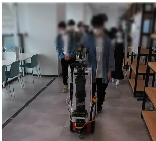
Figure 24. Guiding multiple guests using ASAHl ReBorn. The robot could move with the pace of the head, but it could not wait for other guests behind the head.
