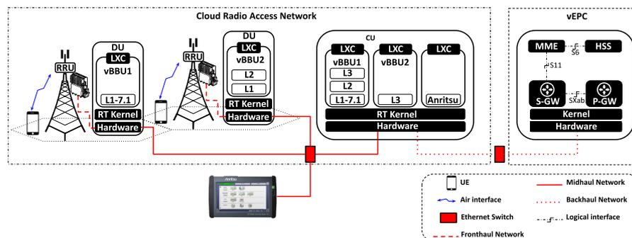
**Figure 8.** Mobile network scenario based on the Cloud-RAN architecture. Deploying two vBBUs with split 7.1 and split 2, respectively. The mobile transport Xhaul is based on switched Ethernet.
