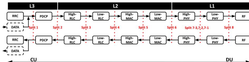
Figure 2. 3GPP functional split of the LTE-BBU functionality [20].
