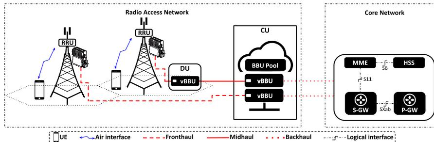
Figure 1. Cloud Radio Access Network architecture.
