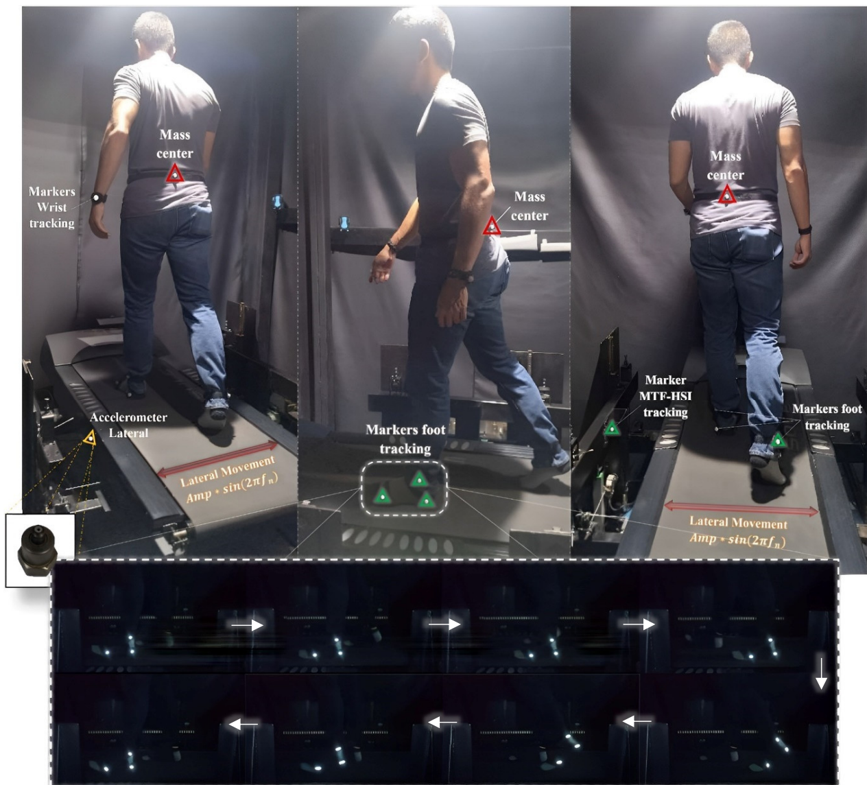
Figure 3. Experimental setup of the human gait test for ST No. 1. Isometric view ( top-left ), lateral view ( top-middle ), and top view ( top-right ). Additionally, a gait cycle ( bottom ).
