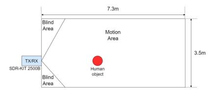
**Figure 2.** Rad-HAR dataset collection environment. There was one subject in the zone. Ancortek SDR-KIT 2500B radar was used to detect the activities.
