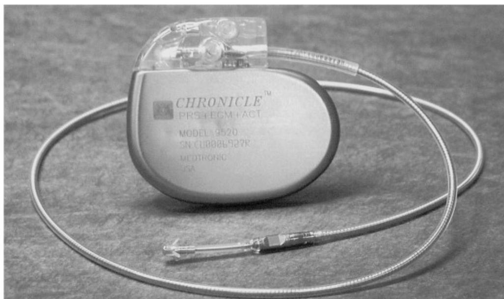
**Figure 3.** The Chronicle IHM System features a single right ventricular lead housing a pressure transducer placed 2.8 cm away from the tined distal tip electrode [45], Copyright 2002, with permission from Elsevier.
