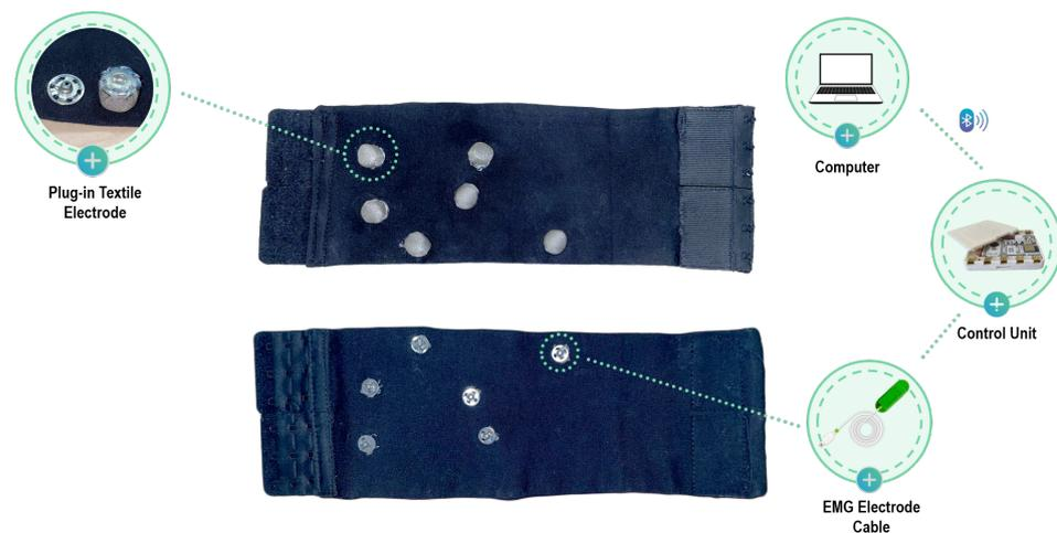
**Figure 4.** Smart textile sleeve: the upper part shows the internal view of the textile electrodes, while the lower part shows the external view connected to the acquisition system.
