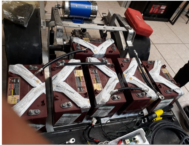
Figure 3. The six TROJAN batteries used to power the electric motor.
