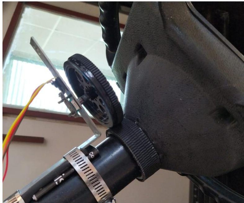
Figure 8. Rotational encoder placed on the steering wheel to measure angular displacement.
