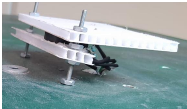
Figure 9. Platform with the magnetometer and accelerometer on top of the vehicle.
