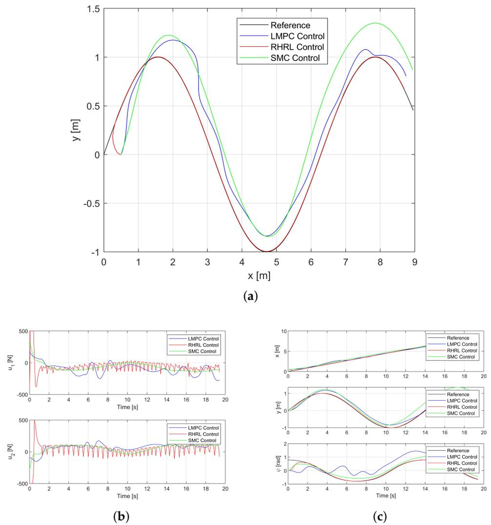
**Figure 6.** The USV trajectory tracking performance in Path I with disturbance. (a) The USV trajectory for Path I. (b) The thrust outputs for Path I. (c) The state trajectories for Path I.
