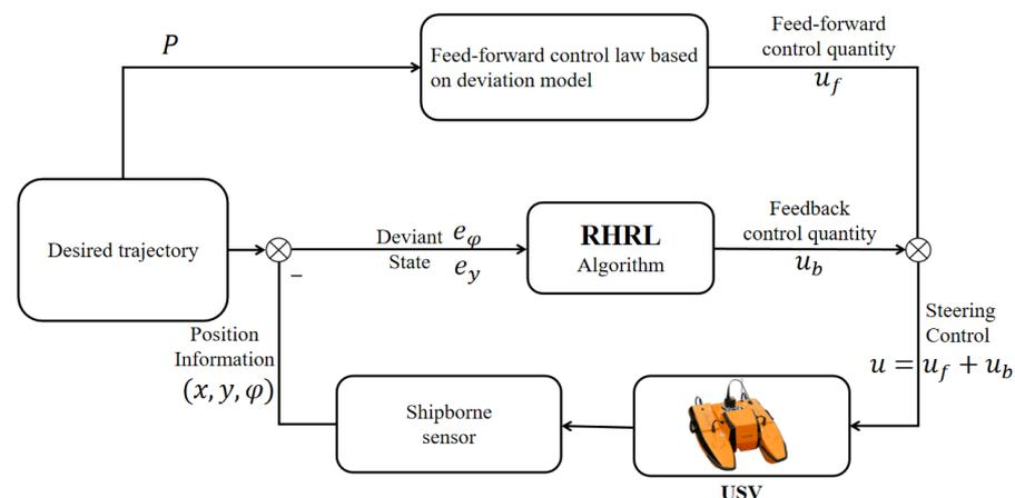
Figure 3. Trajectory tracking control block diagram of the USV.
