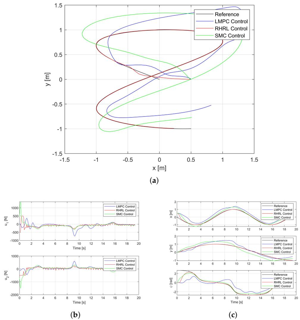
**Figure 7.** The USV trajectory tracking performance in Path II with disturbance. (a) The USV trajectory for Path II. (b) The thrust outputs for Path II. (c) The state trajectories for Path II.
