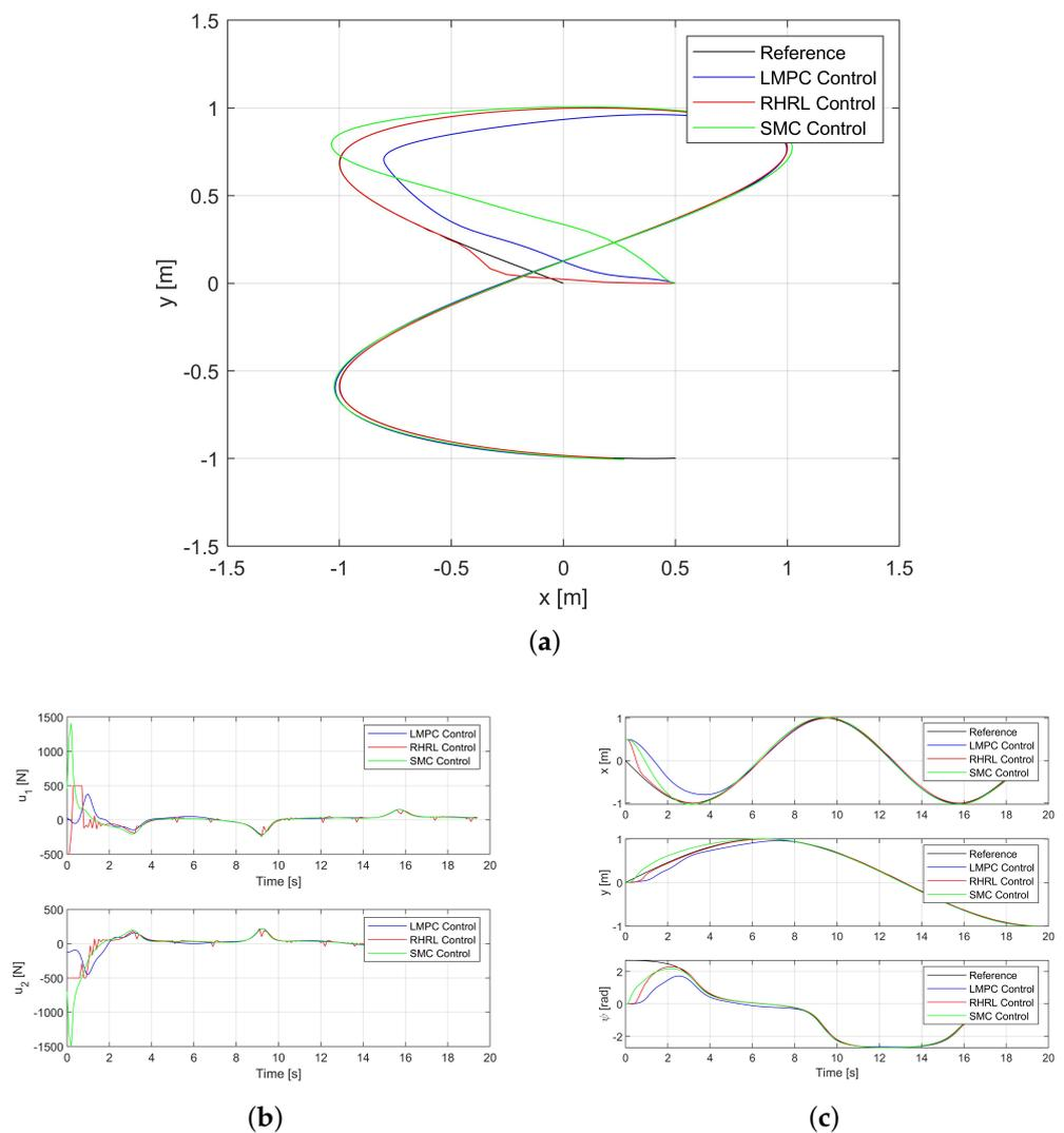
**Figure 5.** The USV trajectory tracking performance in Path II. (a) The USV trajectory for Path II. (b) The thrust outputs for Path II. (c) The state trajectories for Path II.
