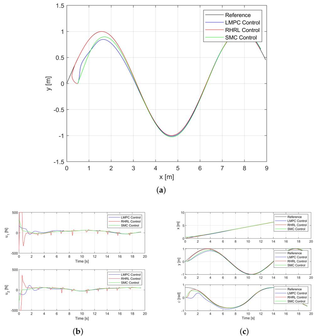
**Figure 4.** The USV trajectory tracking performance in Path I. (a) The USV trajectory for Path I. (b) The thrust outputs for Path I. (c) The state trajectories for Path I.
