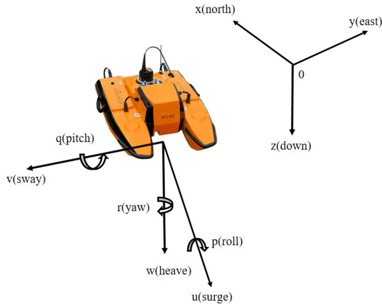
Figure 1. Diagram of the BF (left) and IF (right).
