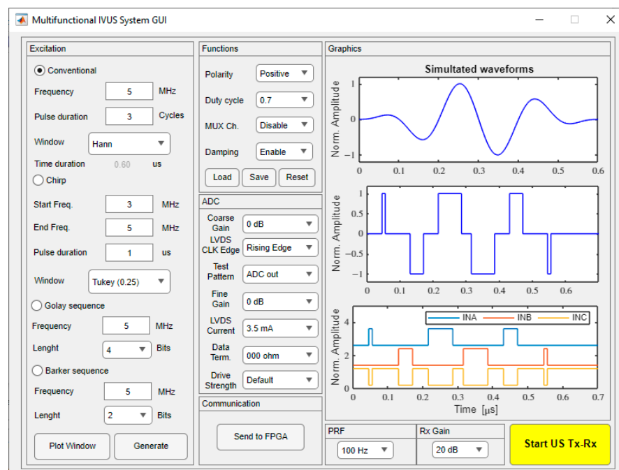
Figure 7. Sample screenshot of the graphical user interface for a three-cycle 5 MHz sinusoidal pulse with a Hanning window and a duty cycle of 0.7.
