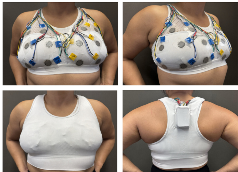
Figure 8. Captured images of the developed system on a participant. Top left: Front-on view of a participant wearing the developed system. Top right: Side-on view of a participant wearing the developed system. Bottom left: Participant wearing a GPS bra over the top of the developed system. Bottom right: Developed system enclosure located within the posterior pocket of the GPS bra.
