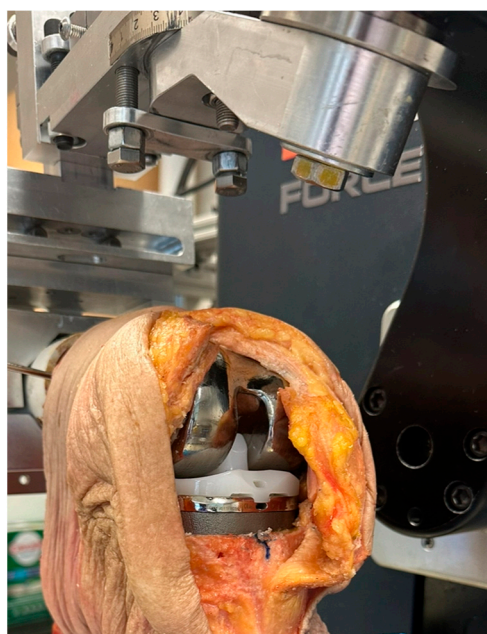
Figure 6. Cadaver knee with implanted TKR mounted on a simulator.
