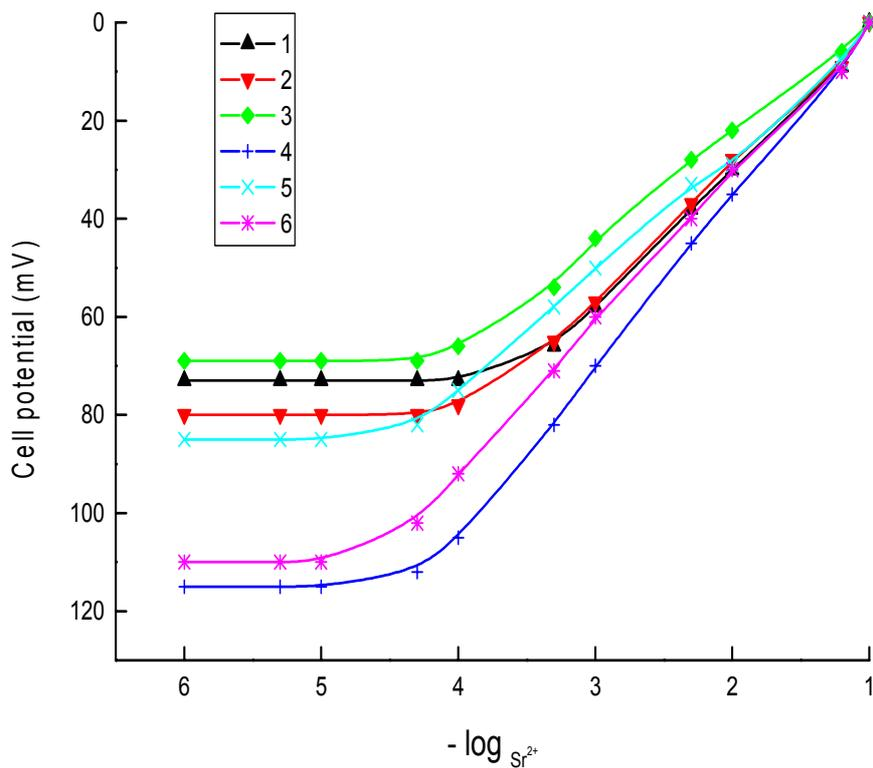
**Figure 1.** Variation of membrane potential with activity of  $\text{Sr}^{2+}$  ions, without solvent mediator (1), with solvent mediators DOP (2), TEP (3), DBBP (4), CN (5) and TBP (6).
