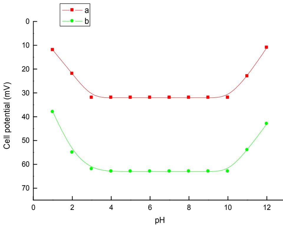
**Figure 2.** Effect of pH on cell potential;  $[\text{Sr}^{2+}] = 1.0 \times 10^{-2}$  (a) and  $1.0 \times 10^{-3}$  M (b).
